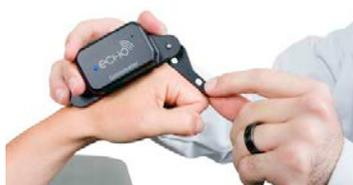
Goniometer orientation for measuring finger MP flexion.
