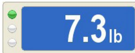
Force and inclinometer measurements are displayed in real time. The dots on the left side of the display indicate instrument connection and battery strength. Green indicates full battery strength.
