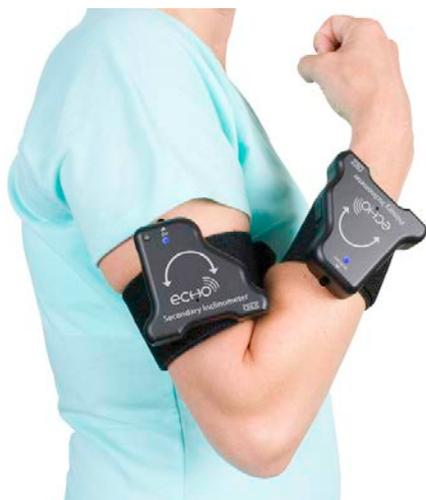
Inclinometer attached at wrist with Velcro strap for dynamic range of motion testing.
