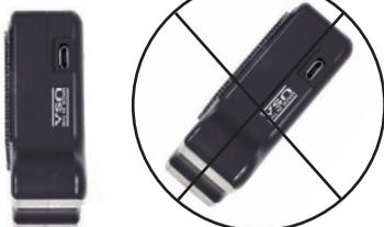
Keep inclinometers in vertical plane when measuring ROM. Tipping the inclinometer (above right) can cause inaccurate measurements.
