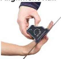
Primary inclinometer with alignment rail attached
