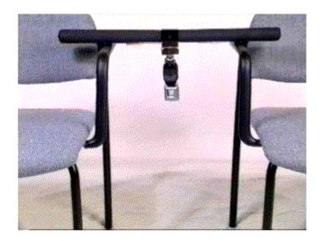
To complete step 2, enter the amount of weight to be added. Attach the weight to the transducer and click on the "Weight Calibrate" button.
