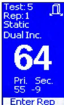
When the Secondary Inclinometer is connected, the LCD will display unique angle measurements for each device, as well as the combined difference.
