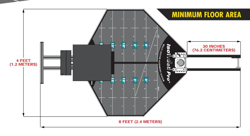
Begin assembly of the IsoTrack Pro Platform in the location where it will be used. A floor space of approximately eight (8) feet by four (4) feet is needed for the assembled IsoTrack Pro. Within that space, 30 inches of open space is needed in front of the IsoTrack Pro Base to ensure that the IsoTrack Pro Multi-Vector Alignment Arm doesn't hit anything during positioning.
